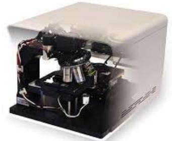
This instrument allows a pathologist located at one location to perform live microscopic review of tissue collected during a surgery at another hospital location – all while the patient is still in the operating room. The tissue is prepared and placed on a glass slide. The slide is inserted into the Mikrosan instrument and a pathologist is called to access the live image.
