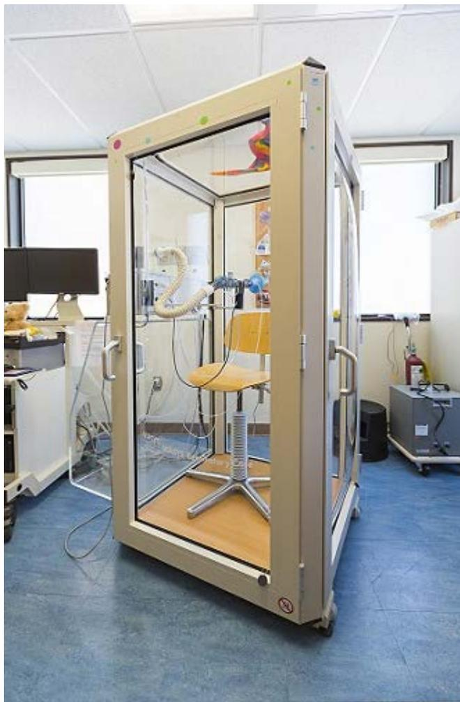
Body plethysmograph used to measure lung volume.
