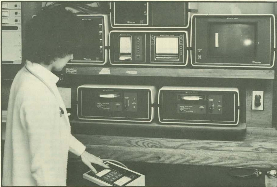
The Coronary Care Unit on Trexler 4 has received new modular bedside and nursing station monitors manufactured by American Optical Company. This sophisticated cardiac monitoring equipment includes eight bedside units capable of constant heart rate and blood pressure monitoring, and respiration monitors which can be moved to the appropriate bedside. The Spectra Central Station, located at the nursing station, monitors all eight patients simultaneously on a computer-type screen. It has print and memory capabilities, when needed, and entirely automatic alarm systems. Jane Babich, R.N., T-4 Staff Nurse, demonstrates use of the monitors.
