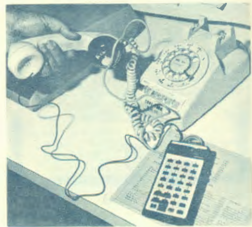
A VIP Communicator ready for telephone transmission in the ER. Note resemblance to miniature calculator.
