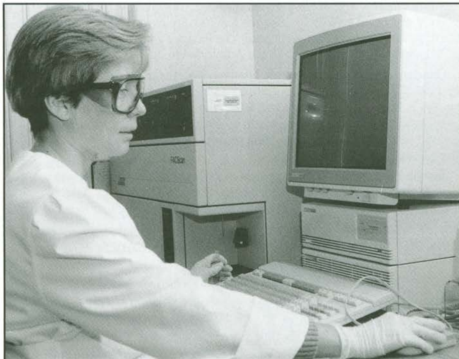
Cynthia Spittle, MT, demonstrates an exotic new device that uses a laser to run high speed counts and sorts of cells of all kinds. Known as Flow Cytometry, it's a vital aspect of service to a diverse range of patients, including AIDS, leukemia and transplants, all of whom have concerns about the relative strength of immune systems.
