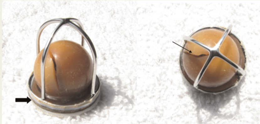
Figure 2 Explanted Starr–Edwards valve. Crack from wear and tear process (thin arrow). The sewing cuff has been stripped (thick arrow).
