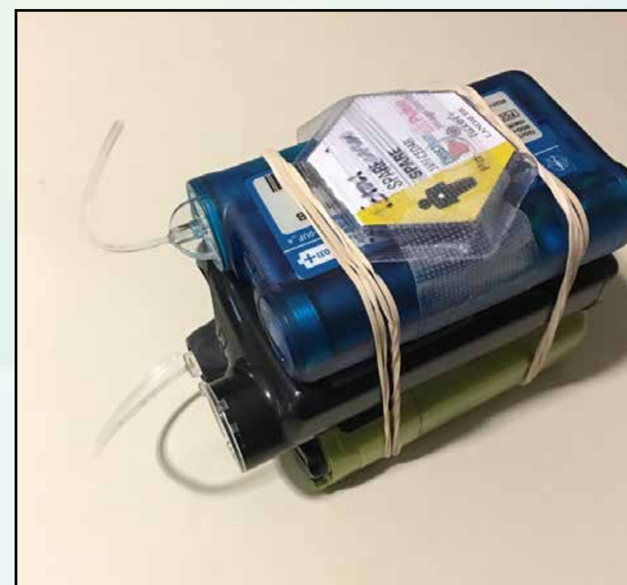
Figure 1: Insulin pump arrangement during radiation.
